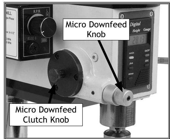
Figure 15. Micro downfeed controls.
